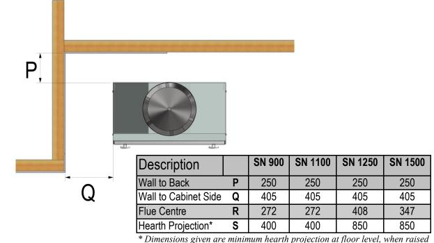
\* Dimensions given are minimum hearth projection at floor level, when raised 400mm above floor level, as the height of the base is, the hearth projection can be 380mm for 900 and 1100 and 450mm for 1250 and 1500.
