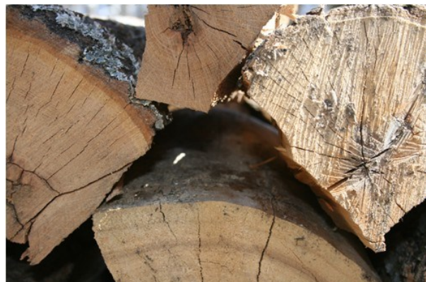
Generally fire wood is cut to 300 to 350mm lengths and split to 150 to 180mm cross section. Note the Season Cracks in the ends.
