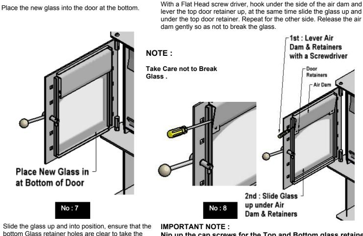
bottom Glass retainer holes are clear to take the cap screws. Fit the bottom glass retainer.
