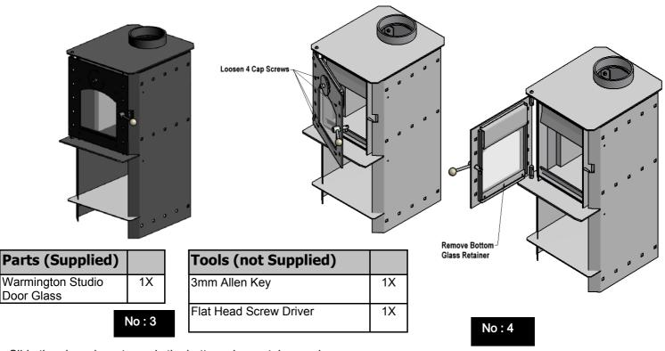
Slide the glass down towards the bottom glass retainer and remove the glass and any shards. May need to Spring the Air Dam with the flat head screw driver.
